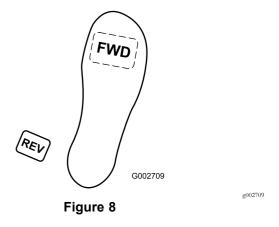
The ground speed is proportionate to how far you press the traction pedal. For maximum ground speed, press the pedal fully while the throttle is in the FAST position. To get maximum power or when ascending a hill, have the throttle in the FAST position while pressing the pedal slightly to keep the engine speed high. When the engine speed begins to decrease, release the pedal slightly to allow the speed to increase.
