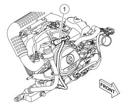
3. Use a spark plug socket to remove the spark plug.
