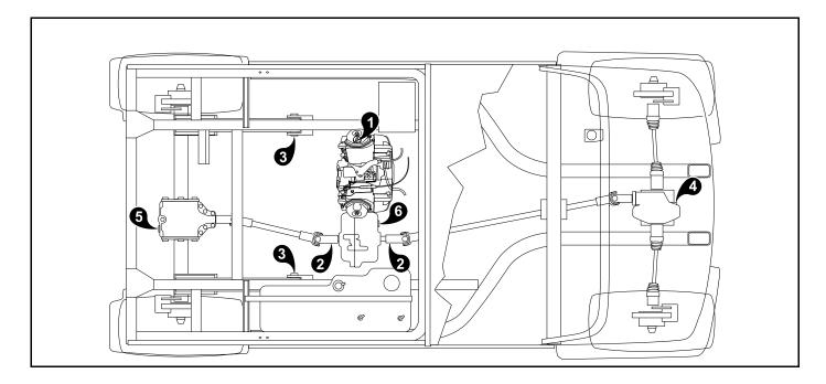
Figure 22 Lubrication Points — Gasoline Vehicles
