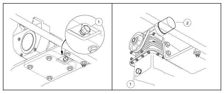
207 Figure 28 Engine Oil Drain Plug and Pan – Gasoline Vehicles
