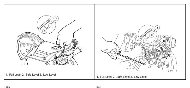
Figure 26 Engine Oil Level Check – Kawasaki Gasoline Vehicles
