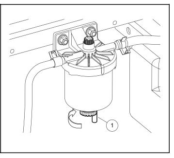
Figure 44 Fuel Filter with Water Separator – Style A
