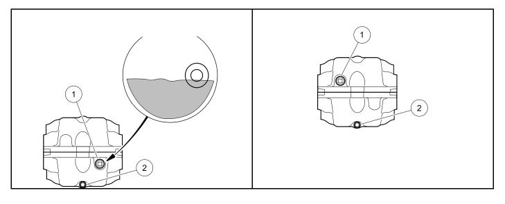
Figure 39 Rear Differential Lubrication Level (2009 to 2011 vehicles)
