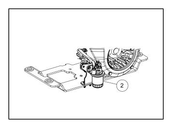
210 Figure 30 Replace Engine Oil Filter – Kawasaki Gasoline Vehicles
