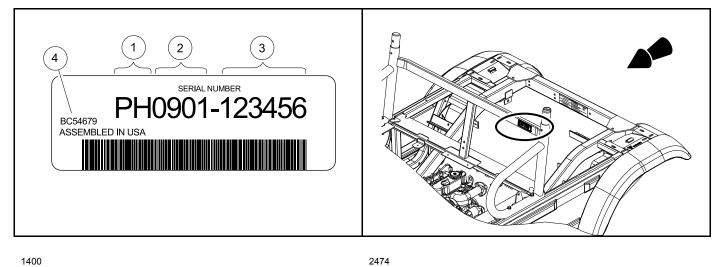
1400Figure 8Serial Number Decal with the Vehicle Build Code
