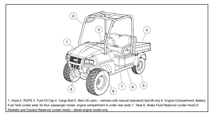
Figure 7 Vehicle Components
