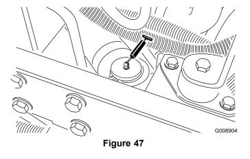
**Note:** If desired, an additional grease fitting may be installed in the other end of the steering cylinder. Remove the tire, install the fitting, grease the fitting, remove the fitting, and install the plug (Figure 48).
