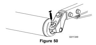
**Note:** Make sure the grease groove in each roller mount aligns with the grease hole in each end of the roller shaft. To help align the groove and hole, there is also an alignment mark on one end of the roller shaft.
