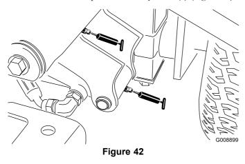
• Right front lift arm pivot and lift cylinder (2) (Figure 43)
