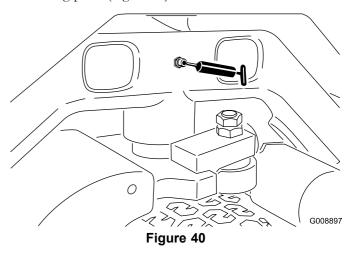
Rear lift arm pivot and lift cylinder (2) (Figure 41)
